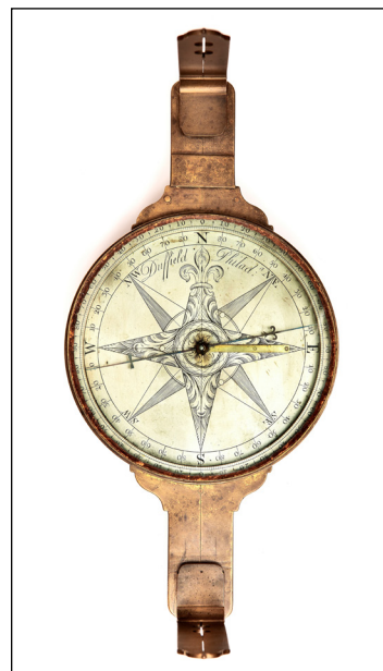
This surveying compass in the collection of the American Philosophical Society dates to circa 1765 and has an unusual quartz pivot bearing at its needle center. Photo courtesy American Philosophical Society.
